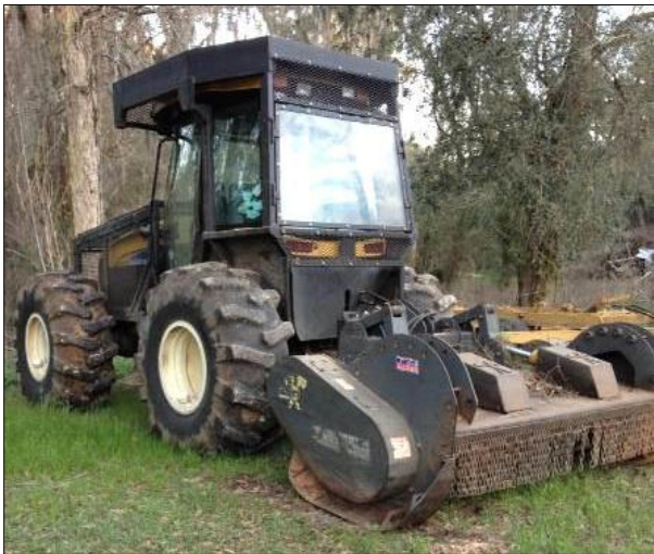
Figure 28: New Holland TV145 with attached Timber Ax allows efficient mowing while minimizing soil disturbance and compaction.
