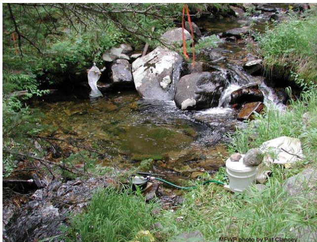
Figure 7. The Montana Bucket trickle system and sentinel fish bag on Cherry Lake Creek. The sentinel fish bag is upstream of the piscicide application point to monitor the effectiveness of the station above the one shown here.
