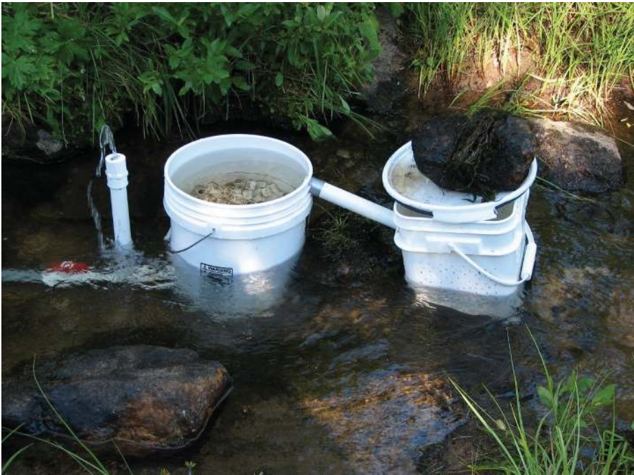
Figure 11. Typical remote streamside incubator (RSI) setup. Water enters via pipe from left, upwells through “gravel” (artificial substrate), and then flows out the top of the RSI. In this set-up, the fry exited the RSI voluntarily and were captured in the second bucket to the right so we could calculate the timing of departure and numbers of surviving fry. Without the trap, the fry would drop directly into the stream.
