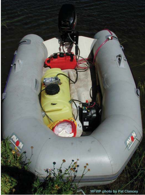
Figure 6. Inflatable raft set-up used to apply Fintrol to Cherry Lake.
