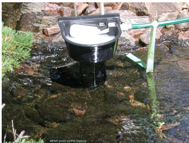
Figure 8. Close-up view of the dog waterer trickling piscicide/stream water mixture into the stream during the Cherry Creek project.
