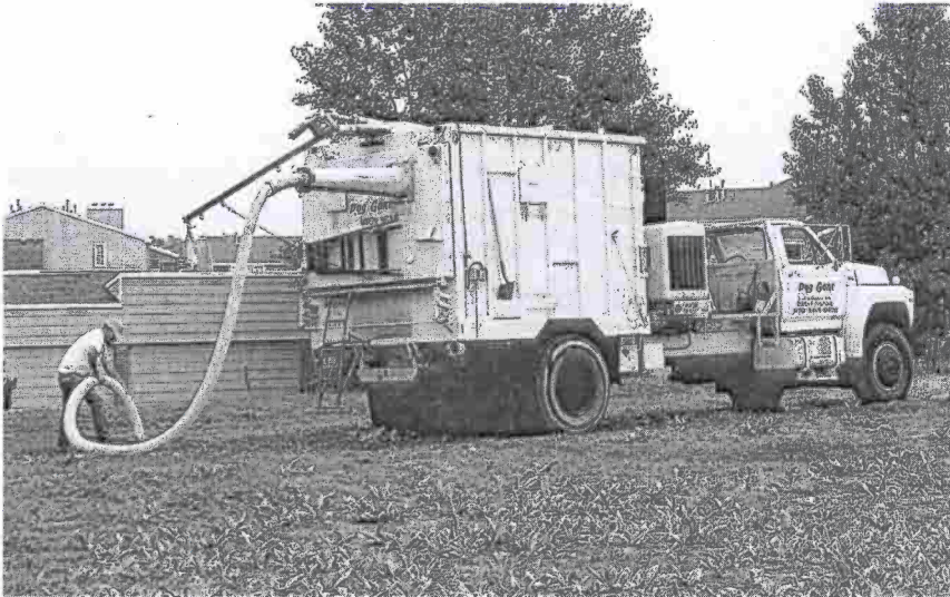
Figure 13.1. Capturing prairie dogs with a vacuum truck. Walls of the truck's receiving chamber are padded with thick foam to deter injuries to prairie dogs as they are pulled through the tube and ejected against the chamber walls. Operators open rear door and climb inside for retrieval. Photo by Joe Truett.
