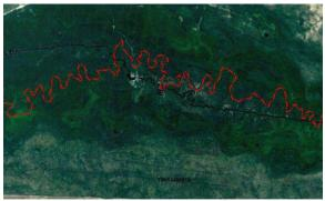
Figure 14.4. Channelized sections of Gordon Creek (dark line) will be realigned to a meander pattern (red line). The creek bed will be raised to elevate groundwater levels and fill wetland basins (shown as lighter shades of green).
