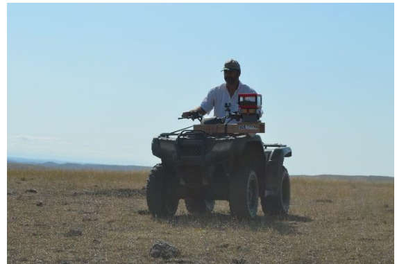
Fig. 2.4. Applying the SPV with a "3-shooter" attached to the front an ATV.
