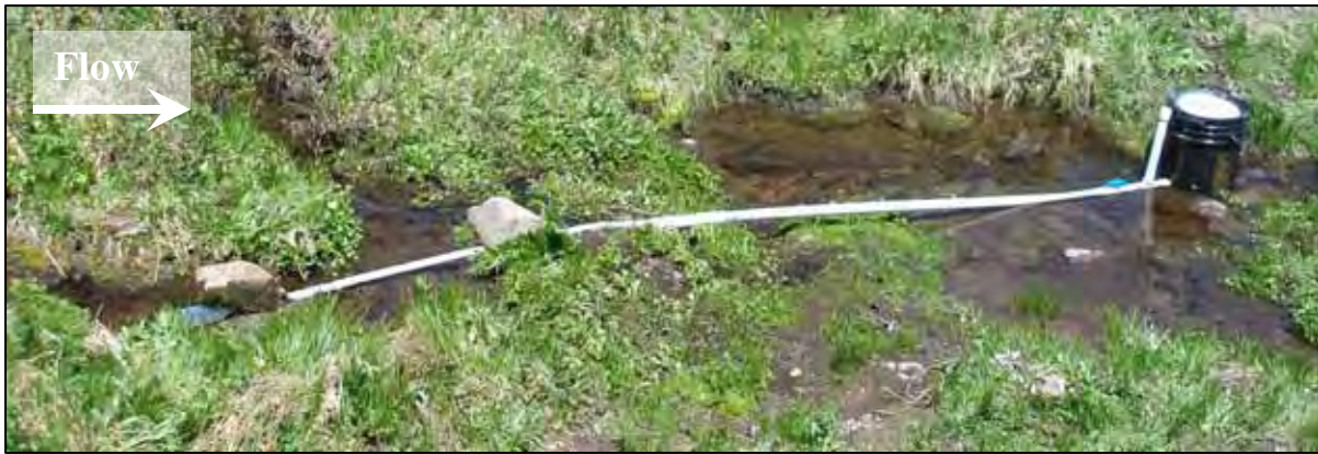
Image 7: RSI setup properly in a small stream, water flowing from right to left.
