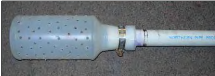
Image 4. Straining bottle attached to end of inlet pipe.
