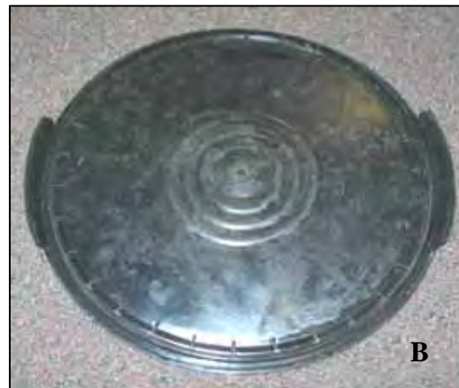
Image 5. A) Bucket with hole drilled into opposite sides. B) Bucket lid with all but two tabs removed; provides easy access into the inner workings.
