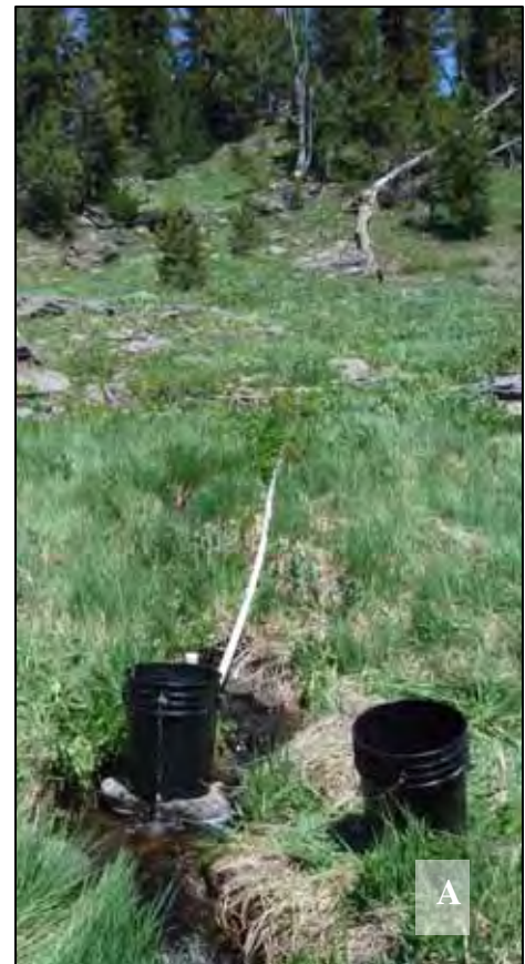
Image 7: RSI setup properly in a small stream, water flowing from right to left.
