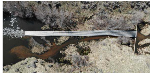
Fig. 8.1. Aerial view of fish barrier, inlet channel (to Green Hollow II), and bypass system.
