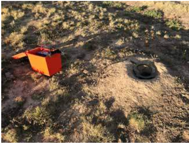
Photo 22.9. Ring-reader in place at prairie dog burrow. The reader is used to detect the individual passive integrated transponder (PIT)-tag number of a reintroduced ferret after it has been observed at a burrow during nighttime spotlighting surveys. This monitoring technique allows researchers to track survivorship of ferrets on a reintroduction site. Each PIT tag is a small radio transponder that contains its own specific code. Photograph: © James N. Stuart.
